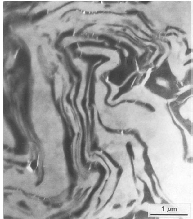
Figure 4 Conical scan dynamic dark field TEM micrograph of Ti-20Y deformation processed to \eta = 5.03 and sectioned transversely. The light grey areas are Ti, and the dark grey areas are Y. The Y phases display numerous fractures across their thickness. Note the similarity in phase shape to the Cu-20Nb specimen shown in Fig. 13.
