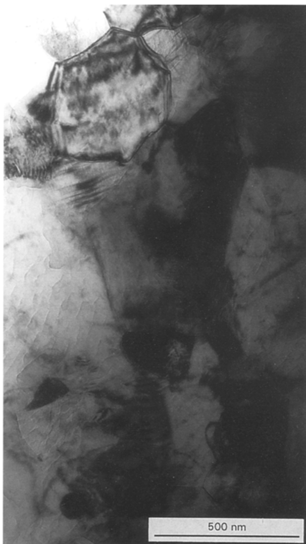
Figure 6 Bright field TEM micrograph of Ti-20Y deformation processed to \eta = 12.2 , annealed at 700 °C, and sectioned transversely. Note the generally equiaxed grains and the lack of plane strain filamentary microstructure as compared to Figs 4 and 5.
