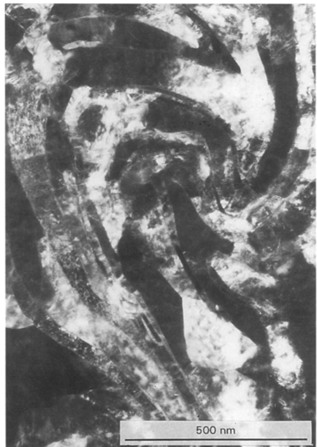
Figure 5 Conical scan dynamic dark field TEM micrograph of Ti-20Y deformation processed to \eta = 7.27 and sectioned transversely.
